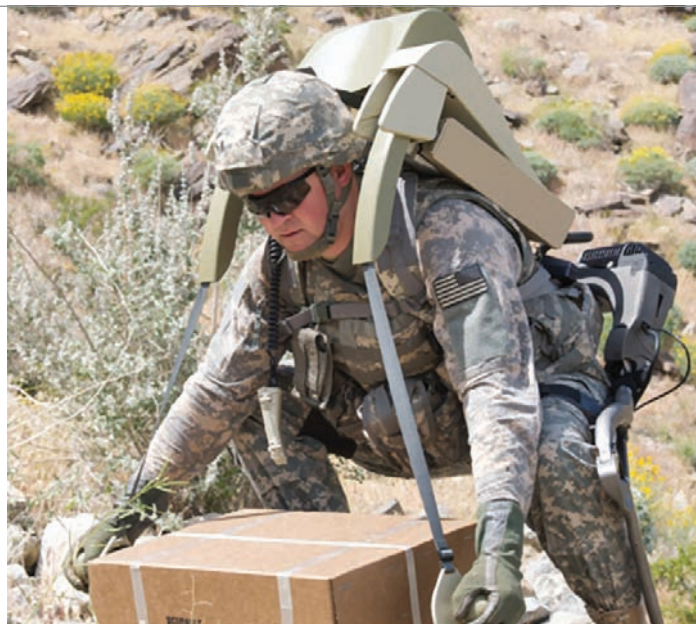
Much of the early research for powered exoskeletons came from military applications such as Lockheed Martin's HULC (Human Universal Load Carrier)
