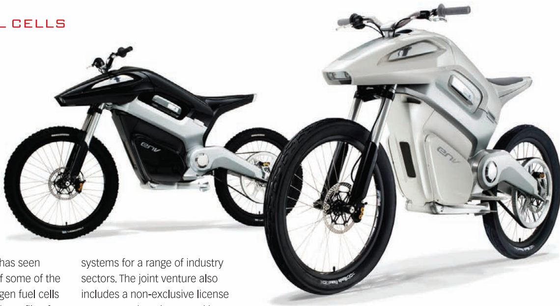
Intelligent Energy developed the ENV (Emissions Neutral Vehicle), a purpose-built, fuel cell-powered motorcycle
