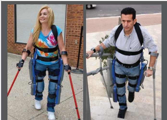
The ReWalk allows users to stand, walk, sit and even climb and descend stairs
